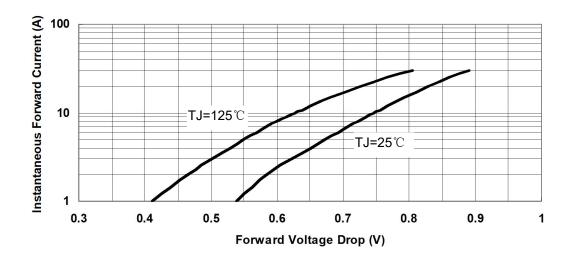
Fig.3-Typical Instantaneous Forward Voltage Characteristics
